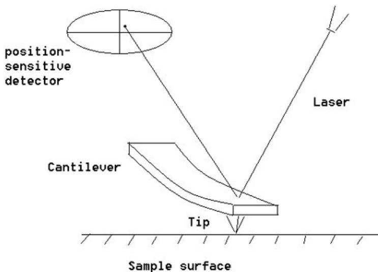
Imaging can be accomplished with either contact mode or tapping (ALSO KNOWN AS NON-CONTACT MODE) mode, and both modes can be used in either air or fluid. In contact mode the tip of the cantilever is in constant contact with the sample surface, whereas in tapping mode the cantilever is not, which consequently reduces sample damages. Due to that, the tapping mode is more commonly used for imaging of soft tissues.
