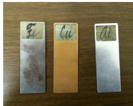
Absorbing plates: Iron (left), Copper (centre) and Aluminium (right)
